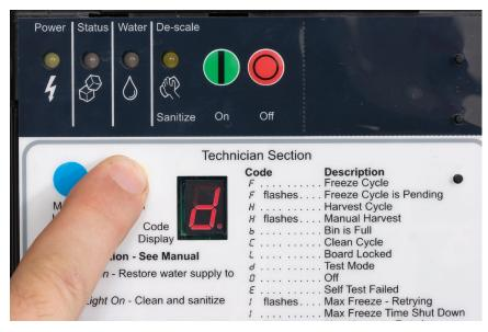
The control can be put into a Test Cycle, where it switches all the loads on and off in a logical sequence. This allows the technician to confirm controller operation of all parts.
