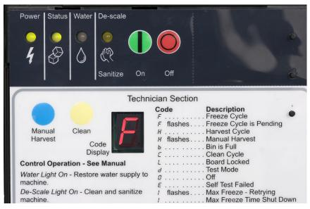
At the beginning of any restart or the first cycle after start up, the controller will display a blinking F.
