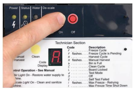
Note: Main Controller Lights and Switches are Duplicated on the Lower Light and Switch Panel
